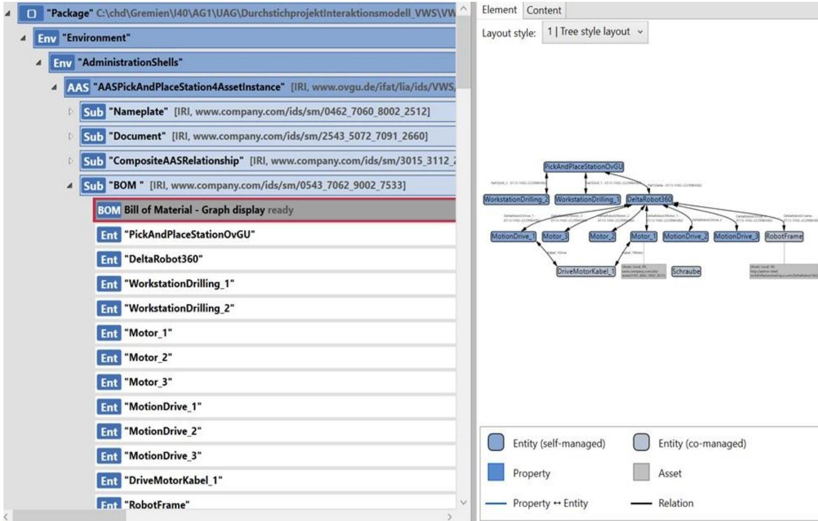
The screenshot shows the AASX Package Explorer on the left and the graph display on the right. The Package Explorer shows a tree structure under 'Env "AdministrationShells"' with a submodel 'BOM' selected. The graph display shows a hierarchical structure of entities and relationships.
